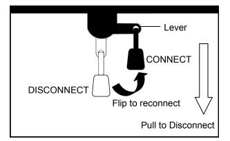
In case of a power failure or door obstruction, PULL EMERGENCY Knob to release door from Opener.
