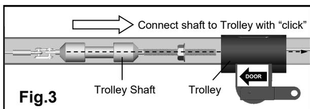
Refer to Fig.3 to connect the Trolley Shaft to the Trolley. Slide both the Trolley Shaft and Trolley towards each other. A "click" will be heard when they are connected.
