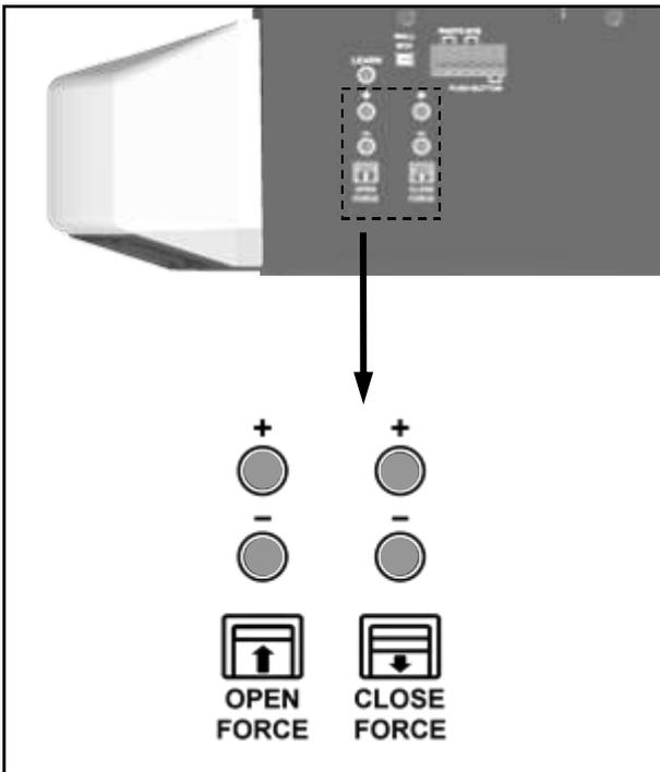
***For safe operation, the force setting should always be set at the MINIMUM FORCE required to run the door.***
